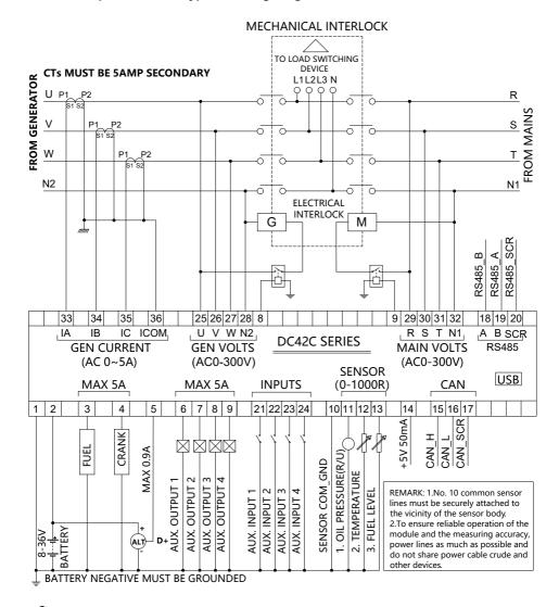
Note: Please don't move battery during running status or it may cause the controller broken!
