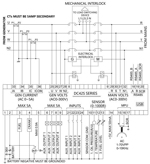
REMARK: 1.No. 10 common sensor lines must be securely attached to the vicinity of the sensor body 2.To ensure reliable operation of the module and the measuring accuracy, power lines as much as possible and do not share power cable crude and other devices
