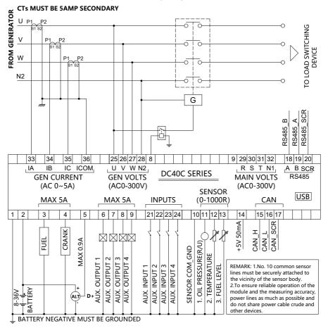
Note: Please don't move battery during running status or it may cause the controller broken!
