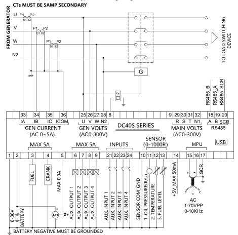
REMARK: 1.No. 10 common sensor lines must be securely attached to the vicinity of the sensor body. 2.To ensure reliable operation of the module and the measuring accuracy, power lines as much as possible and do not share power cable crude and other devices.
