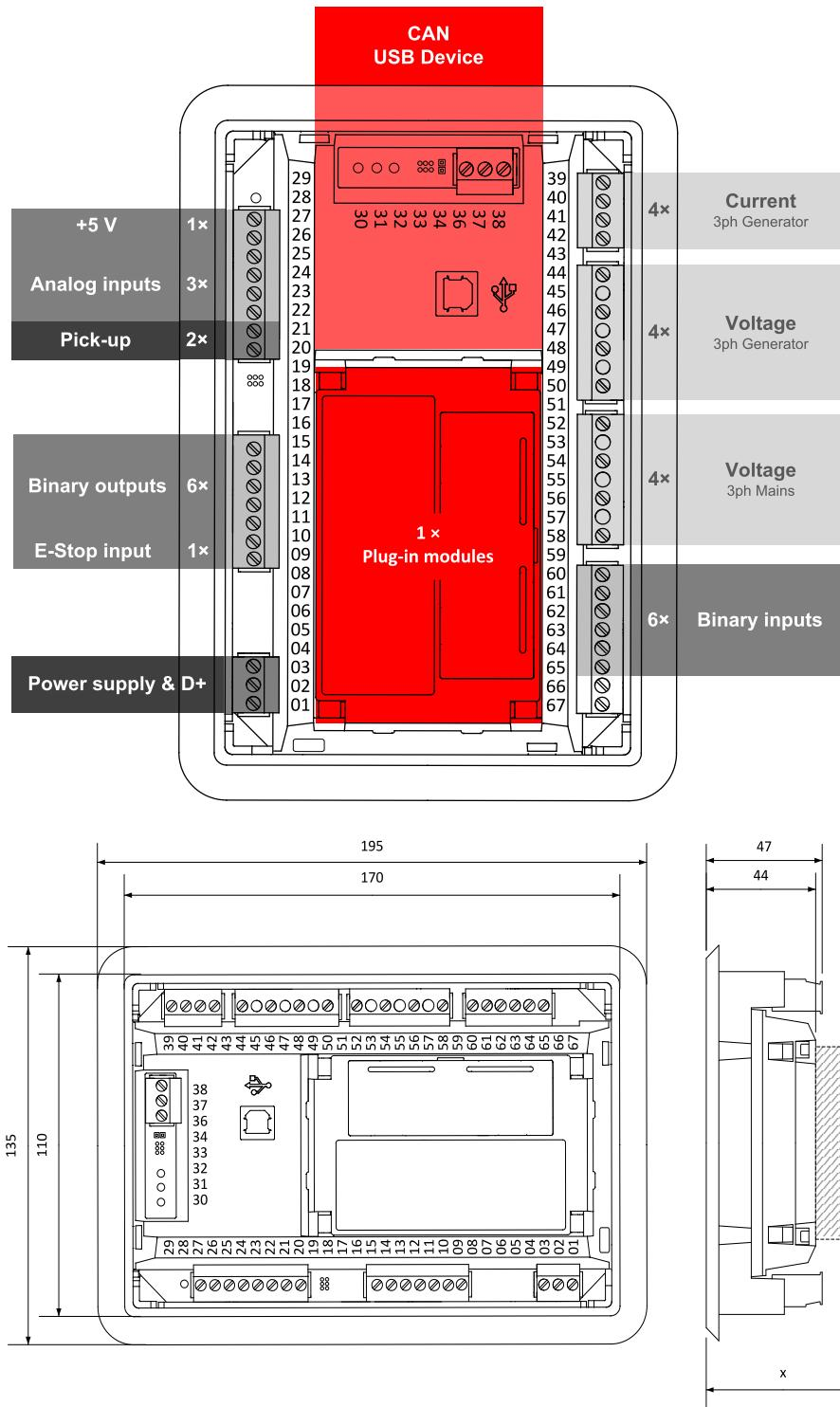
**Note:** The final depth of the controller depends on the selected plug-in module – it can vary between 41 mm and 56 mm. Mind also the size of connectors and cables (e.g. in case of RS232 connector, add about 60 mm more for standard RS232 connector and cable).
